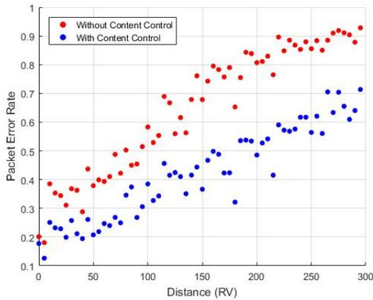
Fig. 6. PER versus Distance for density 125 vehicles/Km
