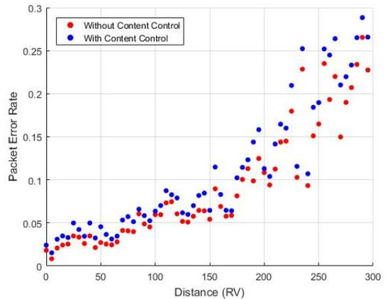
Fig. 5. PER versus Distance for density 25 vehicles/Km
