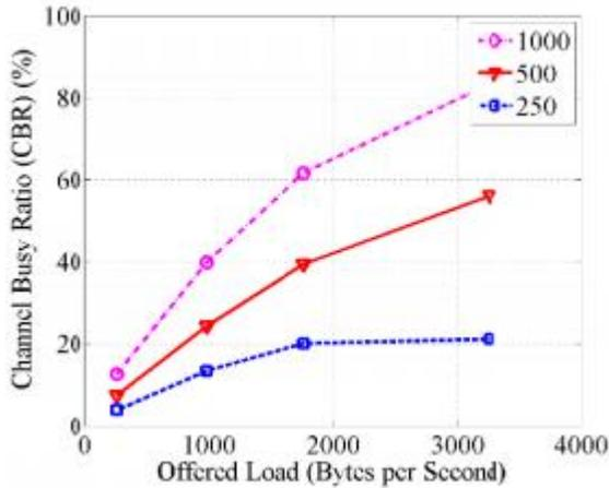
Fig. 2. CBR versus average offered load at 125 vehicles/Km
