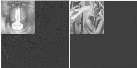
Fig. 5. a, h, v and d components of 1-level decomposition (a) Haar (b) Daubechies Transform
