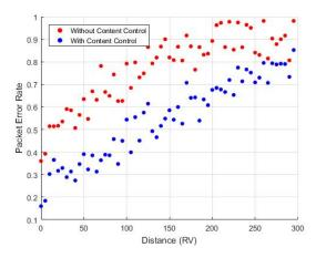
Fig. 7. PER versus Distance for density 250 vehicles/Km
